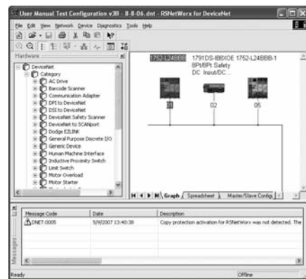
Use RSNetWorx for DeviceNet software to configure all of your DeviceNet devices, including SmartGuard 600 controllers and Guard I/O modules.
